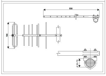
The antenna SA800.7 is designed for base radiostations working in bands of 800-900 MHz. It can be used for receiving and transmitting till 200 W. The antenna has a directional radiation pattern, is broadband and that is why it is suitable for duplex operations.
